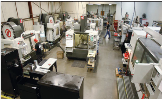
28 Haas 3 and 5-axis milling and turning machines complement the B&B Airparts machining department.
