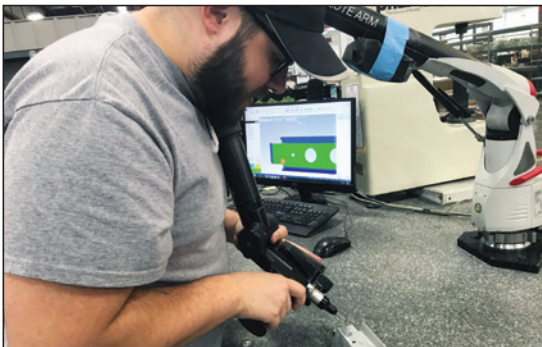
An inspector verifies quality of a part using Verisurf Software and a Romer portable CMM.
