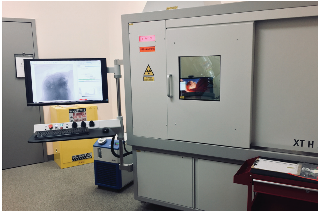
Figure 1. Nikon Metrology XT H 225 ST 225 kV micro-CT system at U of A.
